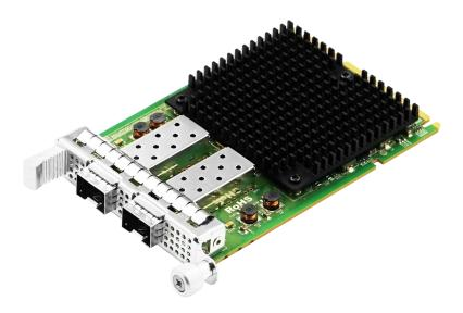
LRES3017PF-OCP is an OCP3.0 SFF dual optical port 25G ethernet network adapter developed by Shenzhen Lianrui Electronics Co., Ltd. based on the intel XXV710 master control solution. The dual ports of the adapter can simultaneously support the self-adaptation of 1/10/25G link rate to meet the flexible use in network environments with different rate requirements, and provide reliable performance in flexible LAN and SAN networks.
